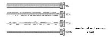
Operating the water heater without the proper anode rod protection will decrease tank life and will void the tank manufacturer's warranty on the tank. To extend the anode life, drain the water from the water heater tank whenever the motor home is not being used. Avoid any extended time of non-use with water in the tank.
