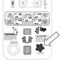
Sewer Tank Flush Inlet on Utility Center
