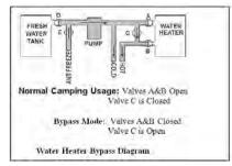
Factory installed 3-valve water heater bypass
