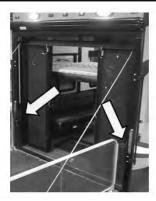
The patio deck comes equipped with mesh end curtains that snap to the door jamb of the rear cargo ramp door (or the side patio door jamb) and to the frame work of the railings. These curtains close off the gap between the railing and the door jamb.
